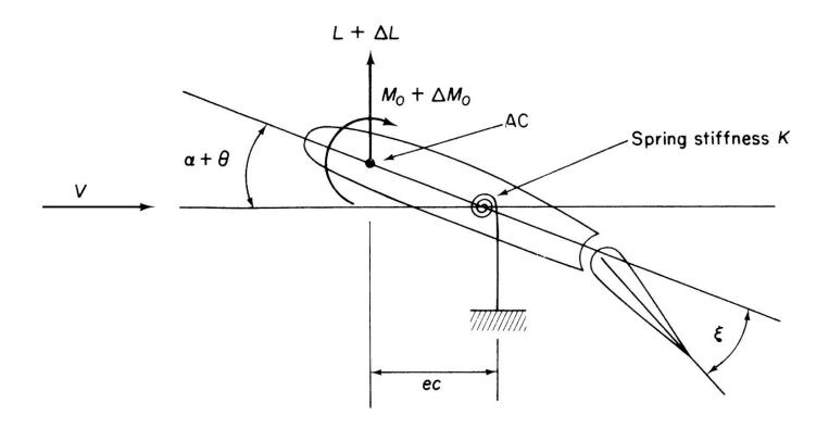
FIGURE 28.5 Aileron Effectiveness and Reversal Speed (Two-Dimensional Case)
