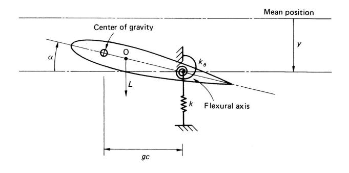
FIGURE 28.10 Flutter of a Wing Section
