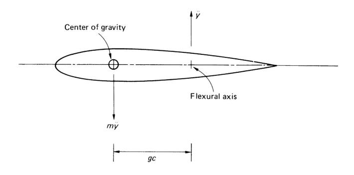
FIGURE 28.8 Inertial Coupling of a Wing
