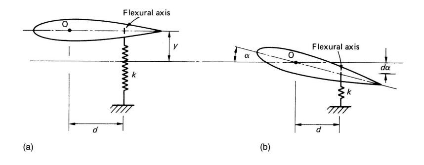
FIGURE 28.9 Elastic Coupling of a Wing
