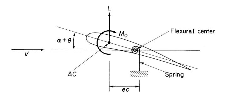
FIGURE 28.2 Determination of Wing Divergence Speed (Two-Dimensional Case)
