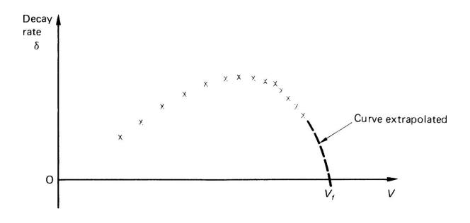
FIGURE 28.11 Experimental Determination of Flutter Speed
