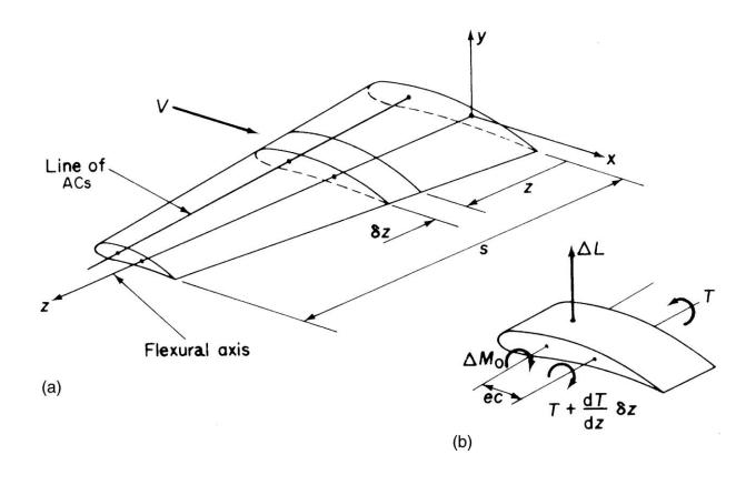
FIGURE 28.3 Determination of Wing Divergence Speed (Three-Dimensional Case)
