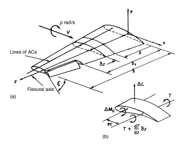
FIGURE 28.6 Aileron Effectiveness and Reversal Speed (Finite Wing)
